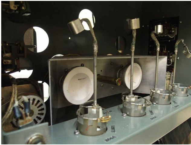
Two heating bulbs R1807 and R1808 only for the look. The round piece at the left behind the interlock switch is the time delay relay K1804 (36 sec.; supply freq. 50Hz).
