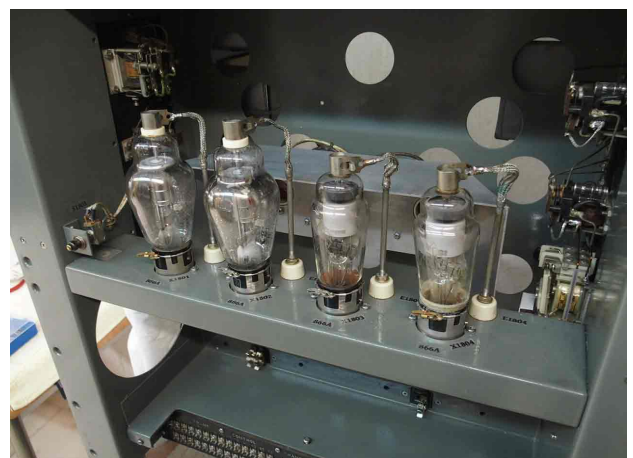
Rectifier tube assembly consisting here of two 866A and two SFR VH55A ( I plan to install four 3B28 rectifiers).
