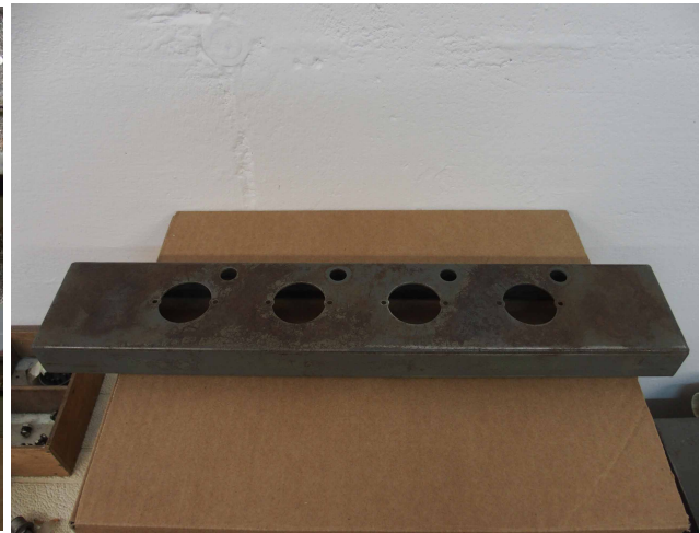
What I called the "MG box" with the Cinch Jones sockets, 115Vac for the motor, and 14Vdc and 28Vdc provided by the generator.
