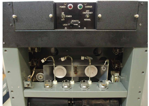
Two heating bulbs R1807 and R1808 only for the look. The round piece at the left behind the interlock switch is the time delay relay K1804 (36 sec.; supply freq. 50Hz).
