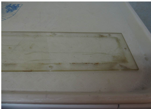
Scratched front plexiglass window before and after cleaning and taking off the scratch first with some steel wool and after that by long polishing with some scratch remover cream for cars.
