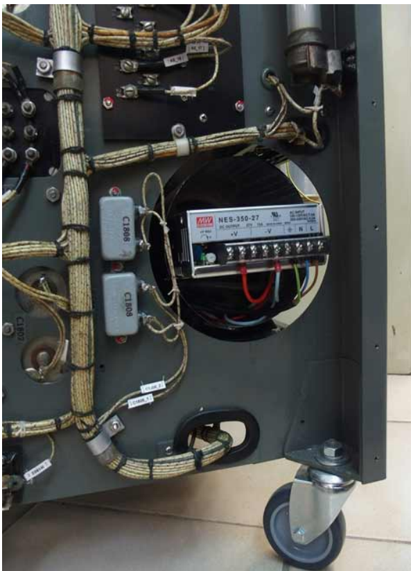
The 28Vdc / 14A power supply hidden in the "generator", place enough for installing a small 12Vdc power supply, but no real interest for ham use.
