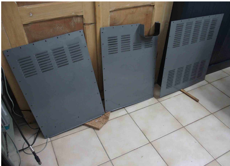
Side and rear covers, (2mm thick !) inside view.
