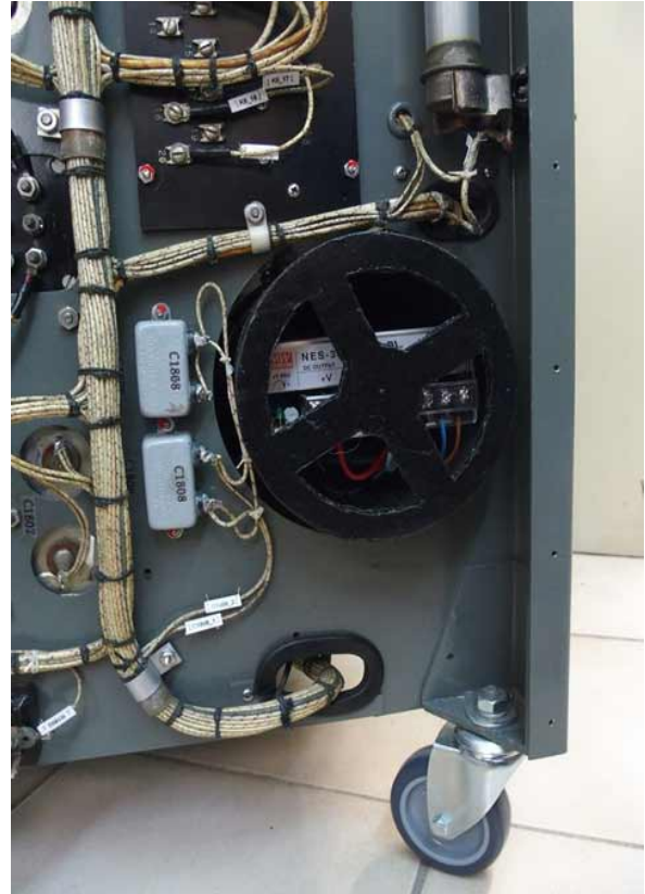
The 28Vdc / 14A power supply hidden in the "generator", place enough for installing a small 12Vdc power supply, but no real interest for ham use.
