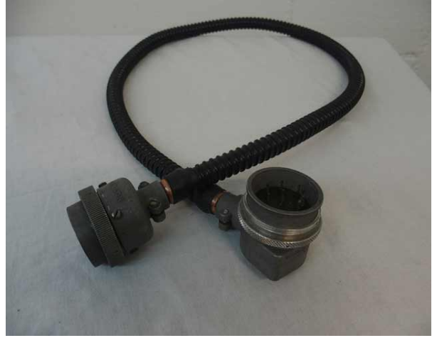
ART-13 / PSU cable, over-insulated HV wire and oversized 28Vdc wires . The cable is longer than the original one, so the transmitter can be positioned in a larger area.
