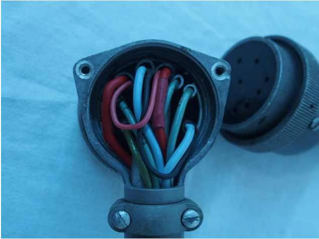
ART-13 / PSU cable, over-insulated HV wire and oversized 28Vdc wires . The cable is longer than the original one, so the transmitter can be positioned in a larger area.
