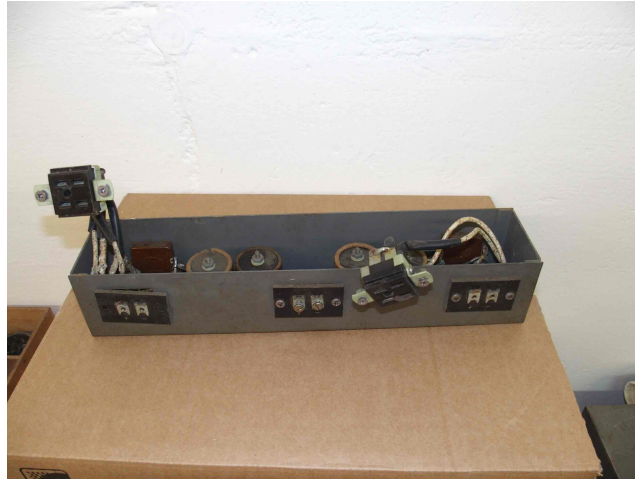
What I called the "MG box" with the Cinch Jones sockets, 115Vac for the motor, and 14Vdc and 28Vdc provided by the generator.
